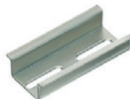
TS 35/15 mm according to EN 50022 (s = 1.5 mm)
