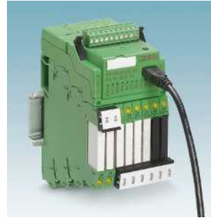
Programmierbares Logikrelaisystem PLC logic
