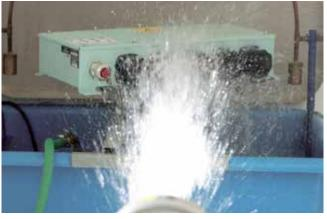
VARITAIN are subject to diverse quality tests, including impact stability, salt water resistance and diverse water ingress protections
