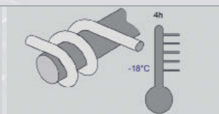
Flexibilitäts-Test CSA-C 22,2 Nr. 227, 3-M91 Flexibility test CSA-C 22,2 No. 227, 3-M91
